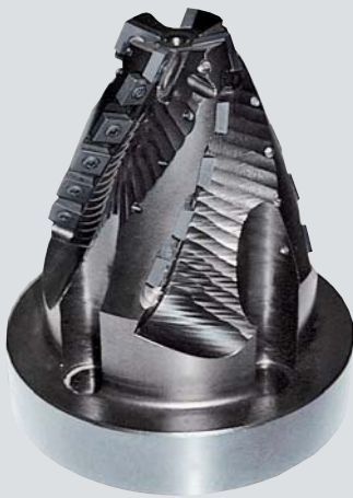
Zahnform-Fingerfräser (Vorfräser) m 48-Stub, E \sphericalangle 20°, Ø 150 x 180 mm Länge, 22 Wendepplatten End mill type gear cutter (roughing cutter) m 48-stub, 20° p.a., 150 dia. x 180 mm length, 22 indexable carbide inserts
